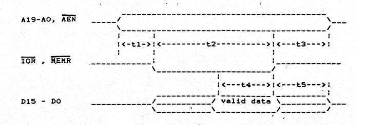
FIGURE 7-1. HOST PROGRAMMED I/O OR BIOS ROM READ TIMING DIAGRAM
