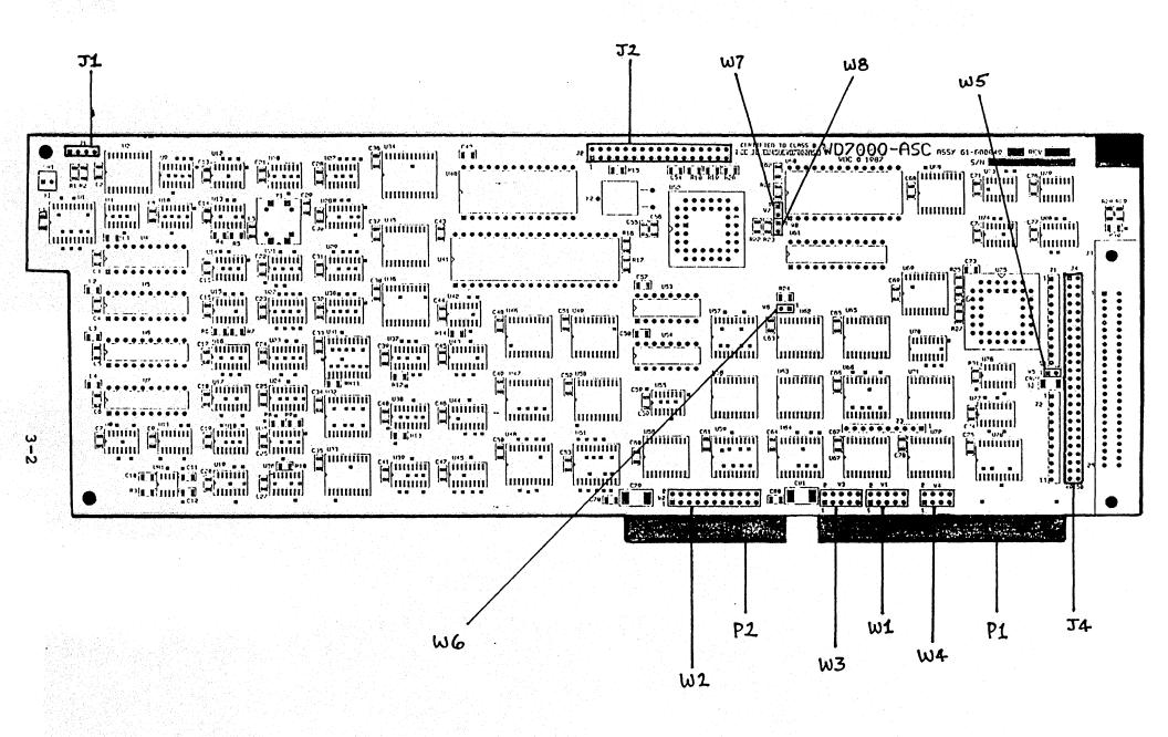
FIGURE 3-1. WD7000-ASC BOARD CONNECTORS AND JUMPER LOCATIONS
