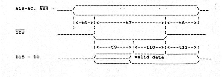
FIGURE 7-2. HOST PROGRAMMED I/O WRITE TIMING DIAGRAM
