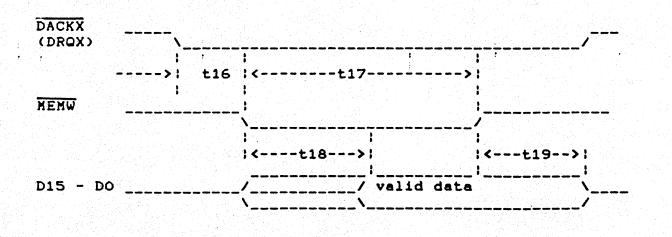
FIGURE 7-4. HOST DMA I/O WRITE CYCLE TIMING DIAGRAM
